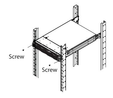
Figure 13: Optional screws to secure chassis to rack.
